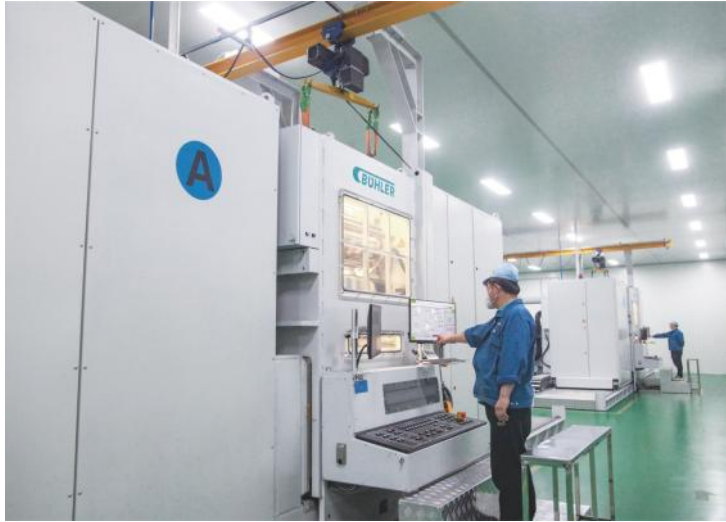
引进德国布勒莱宝光学高真空卷绕式电容用镀膜机 2 台 Germany Buhler Leybold brand of vacuum coating plant: 2 sets.
