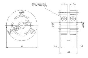
Spring washer-type coupling, three part, plug-in (8.0000.1402.XXXX)
