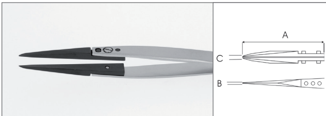
72ZJ.SA A 1.2" 30mm - B 0.007" 0.2mm - C 0.016" 0.4mm replaceable tips set code: A72ZJ
