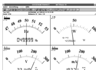
Multimeter-display for up to 4 channels
