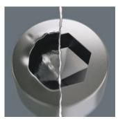
Hexagon screws can endure a problem because the contact surfaces delivering the power from the conventional tool, transferred to the screw via very surface small areas. The consequence: the screw can become damaged (rounding out). Hex-Plus tools have a greater contact surface that prevents this from happening! At the same time, as much as 20 % more torque can be applied. Good to know: Hex-Plus tools fit into every standard hexagon socket screw!
