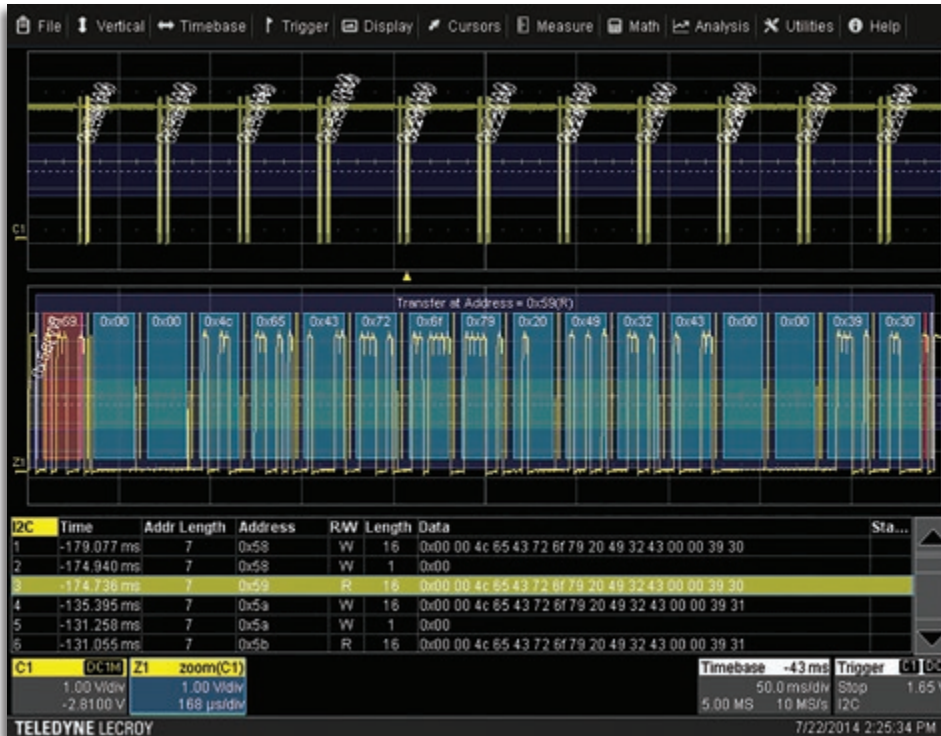
View decoded protocol information on top of physical layer waveforms and trigger on protocol specific messages.
