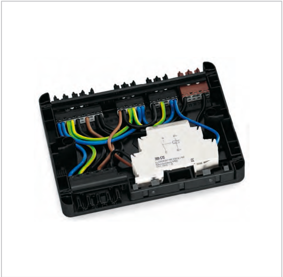
Solid conductors are terminated via push-in termination, while stranded and fine-stranded conductors are inserted using an operating tool.
