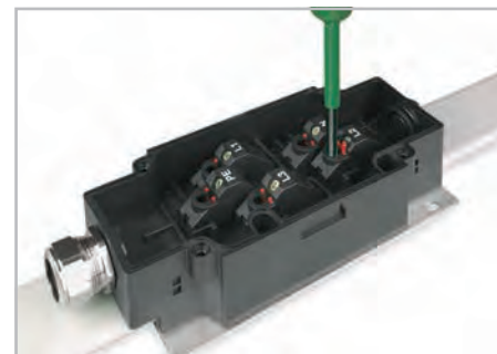
Red contact clips confirm that the contacts are made correctly when they are flush with the terminals.
