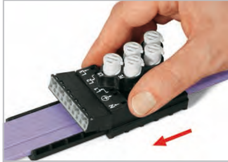
Mount IDC module flush with the base. Should the IDC module jam during mounting, turn the upper part by 180° and remount it.
