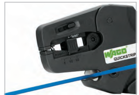
Cutting a conductor.
