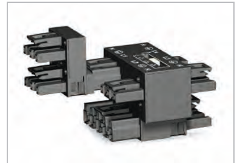
An additional h-distribution connector doubles L1. This results in the following connection options: L1/L1/L2/L2/L3 with jumper in position L2 L1/L1/L2/L3/L3 with jumper in position L3
