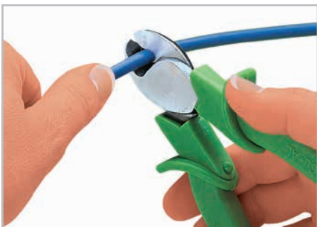
Cutting a cable.
