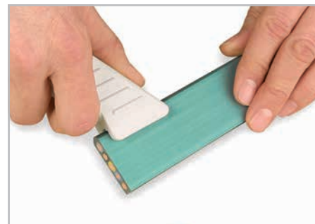
Cut both sides of the outer insulation of the flat cable using a stripping knife (observe 30 mm of cutting length).
