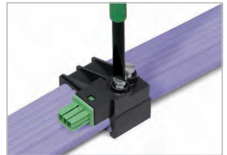
Contact is made with the flat cable by tightening the screws. Observe 1 Nm of tightening torque!
