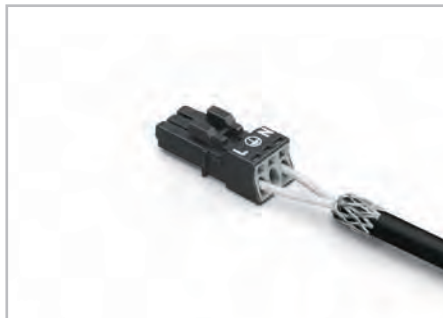
Apply the shield to the rubber cable. Strip length, outer insulation = 30 mm Shield length = 8 mm
