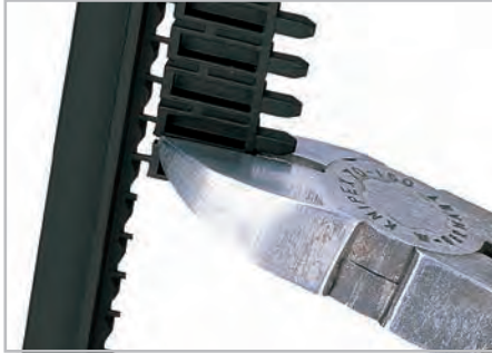
Remove unrequired areas from the sidewalls.
