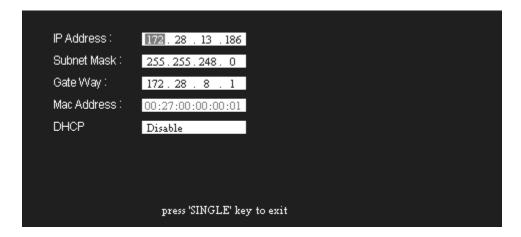
3. Enter an **IP Address**, **Subnet Mask**, and **Gate Way**. Enter values by selecting each segment and turning the Adjust knob until the desired number is reached. Press the top soft key to jump to the next field or press the Adjust knob to tab to the next segment of the current field. Leave DHCP disabled.
