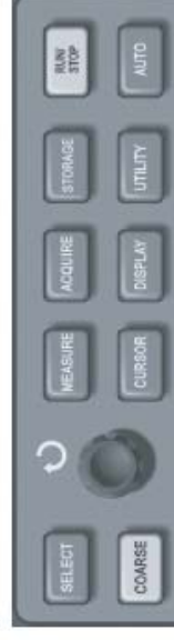
Figure 2-22 Function key for the sampling system (storage).
