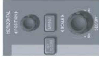
Figure 1-10 Horizontal control zone on the front panel
