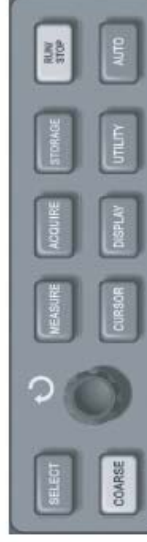
Figure 2-29 Function key for the sampling system (cursor).
