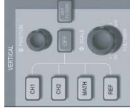
Figure 1-9 Vertical control zone on the front panel
