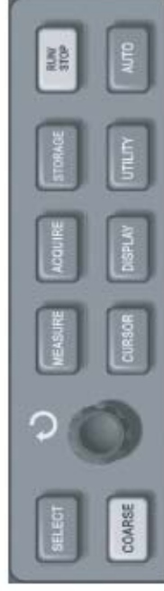
Figure 2-28 Function key for the sampling system (auto measurement).
