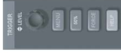
Figure 1-11 Trigger menu on the front panel
