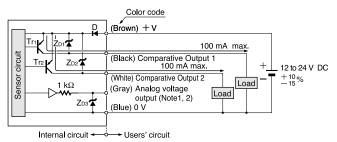
Notes:1) When using the analog voltage output, take care to connect external device of proper input impedance. Also, when a cable extension is used, voltage drop due to cable resistance should be taken into account.
