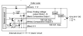
Notes:1) When using the analog voltage output, take care to connect external device of proper input impedance. Also, when a cable extension is used, voltage drop due to cable resistance should be taken into account.
