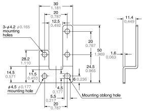
Material: Cold rolled carbon steel (SPCC)
