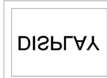
Fig. 9.9 Vertical reverse (U/D: Low; L/R: High)
