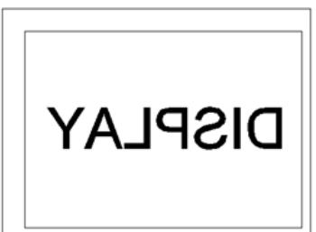
Fig. 9.10 Horizontal reverse (U/D: High; L/R: Low)
