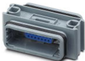
D-SUB coupling, shell size 2, socket, gender changer, shielded, connection direction straight, IP67 degree of protection
