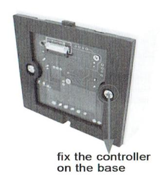
(4) use your hand gently pull down the cable seat lock according to step 2, plug the cable into cable seat, press the lock, and mount the cable of panel on the base, as shown below:
