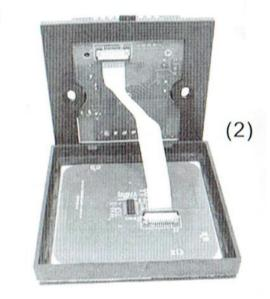
(2) remove the cable. Pull the locking of the terminal transposon, and then you can slowly remove the cable, as shown below:
