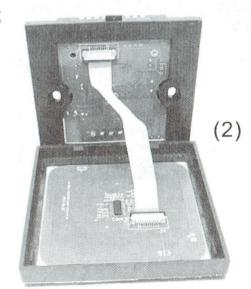
(2) remove the cable. Pull the locking of the terminal transposon, and then you can slowly remove the cable, as shown below:
