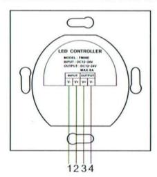
**INPUT:** 1 and 2 are power input pins, input voltage range is 12-24V; 1 is negative and 2 is positive.
