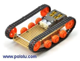
Tank-style chassis built using the Tamiya 70100 track and wheel set, Tamiya 70098 universal plate set, and Tamiya 70097 twin-motor gearbox kit.
