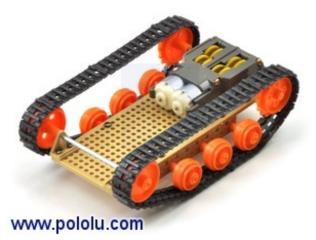
Tank-style chassis built using the Tamiya 70100 track and wheel set, Tamiya 70098 universal plate set, and Tamiya 70097 twin-motor gearbox kit.
