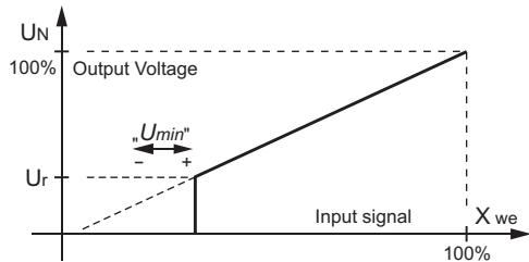
You can set the initial value of the voltage  $U_r$  (eg. starting voltage for the motor)
