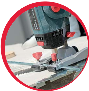
Guide for longitudinal cutting
