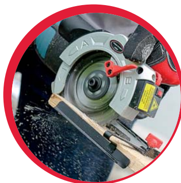
Supporting foot and guide for longitudinal cutting
