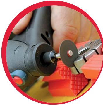
Cutting with an abrasive disc
