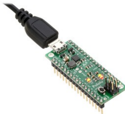
A-Star 32U4 Mini SV with soldered headers and connected USB cable.
