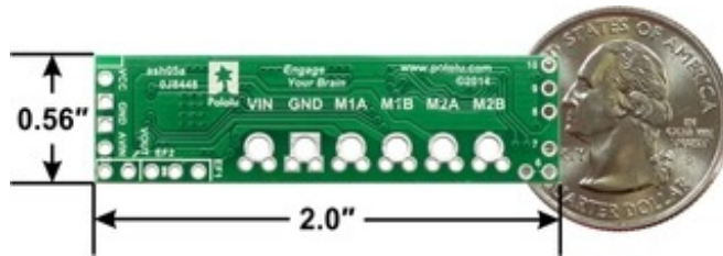
Pololu A4990 Dual Motor Driver Shield for Arduino, top view with dimensions.
