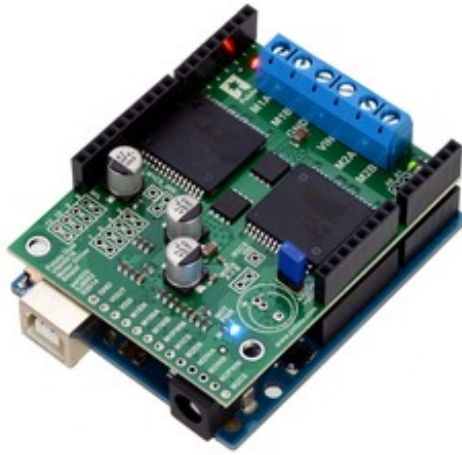
Pololu dual VNH5019 motor driver shield, assembled and connected to an Arduino Uno R3.
