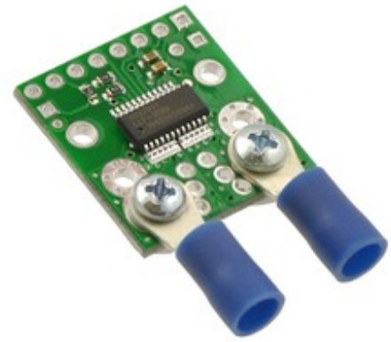
ACS709 current sensor carrier with solderless ring terminal connectors (not included).
