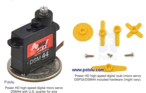
Note that, as with most hoy servos, stalling or back-driving this servo can strip its gears.
