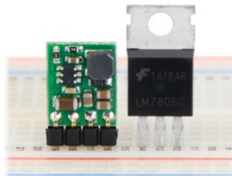
Pololu step-down voltage regulator D24VxTx next to a 7805 voltage regulator in TO-220 package.
