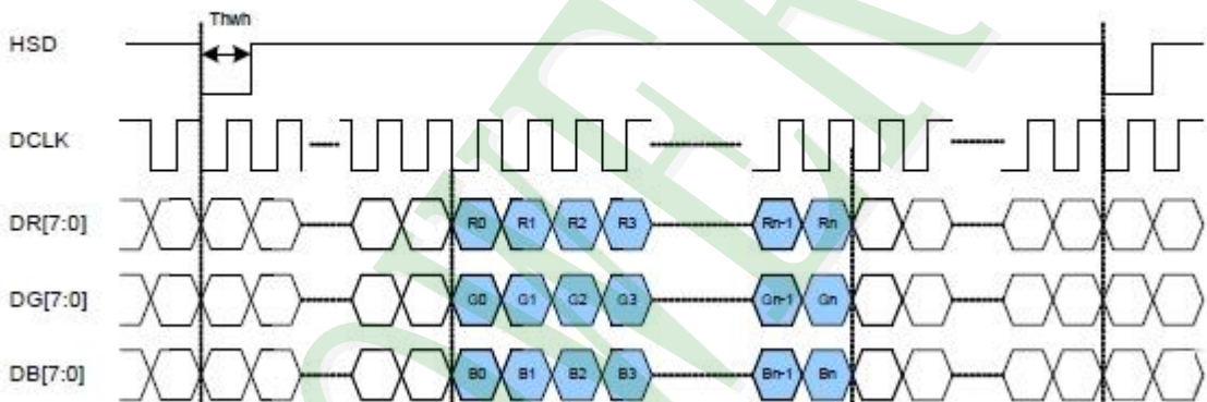
Parallel RGB Mode Data format
