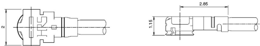
Figure 12-2: ORG1408 receptacle mechanical drawing
