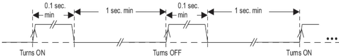
Figure 7-1: ON\_OFF timing
