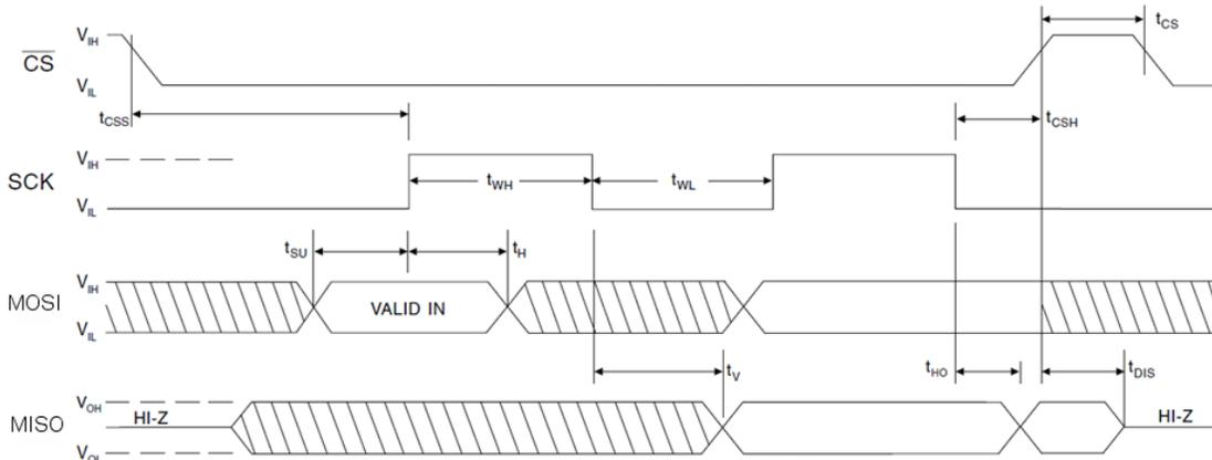
Figure 7-3: SPI timing
