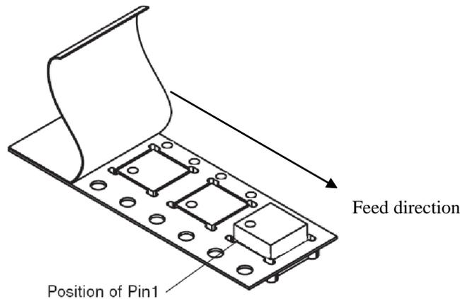
Figure 11-2: Module position
