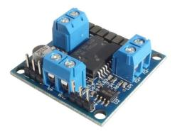
The *DC Dual Motor Driver 30V 4A V2* allows to indipendently drive two DC motors, controlling both velocity and direction.
