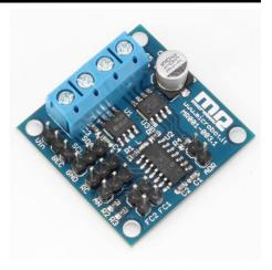
The *Easy Motor Controller* allows to control the speed and the direction of rotation of a DC motor through three different possible inputs: analog (potentiometer), radio control RC, I2C digital communication.
