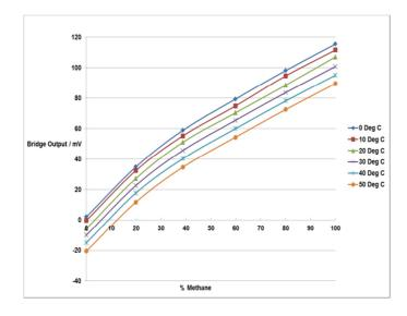
The responses exhibit a quadratic behaviour and tests have shown that a 3 point calibration at 0, ~40 & 100% Methane will generate factors which will meet the requirements of EN 60079-29-1 2007 part 5.4.3.2 i.e. within  $\pm$ 3% Methane or  $\pm$ 5% of indication
