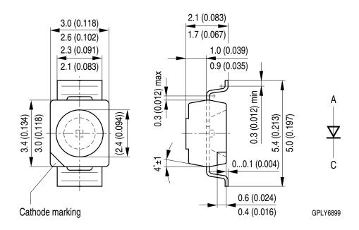
Approximate Weight:34.0 mgPackage marking:CathodeCorrosion test:Class: 3B
