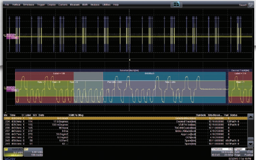
View color-coded overlays on top of the analog waveform for quick identification of the ARINC 429 word. Click on the table to zoom the ARINC 429 word to view individual bits.
