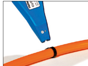
Bring the tool perpendicular to the tie...
