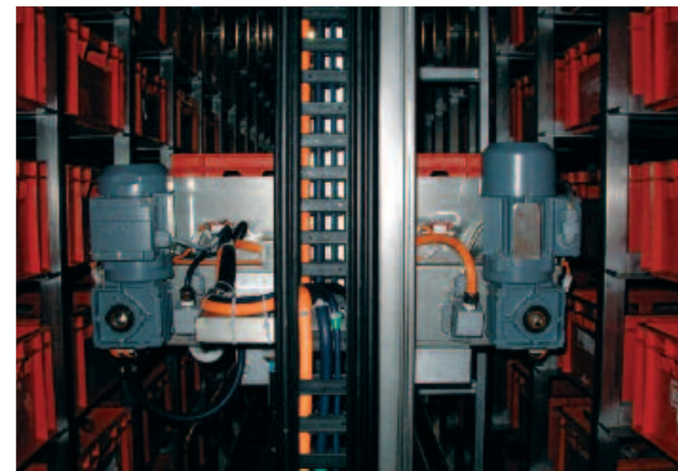
Control cable chainflex® CF10 in storage and retrieval units for high-bay warehouses. e-chain®: System E2 medium
