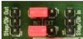
Figure 3.7 Jumper setting for TMC4210 selection.
