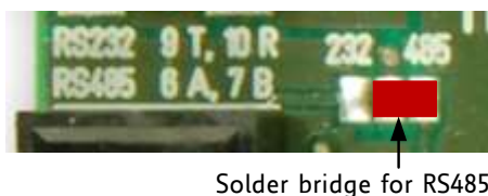
Figure 3.4 Solder bridges for RS232 and RS485
