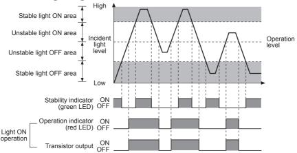
\*\*The waveform of 'Operation indicator' and 'Transistor output' are for Light ON operation.
