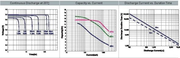
\*\* This data was made on basis of nominal capacity for the purpose of enabling users to forecast approximate life time. In order to calculate precise life time under various environments, we recommend you to consult Vitzrocell.
