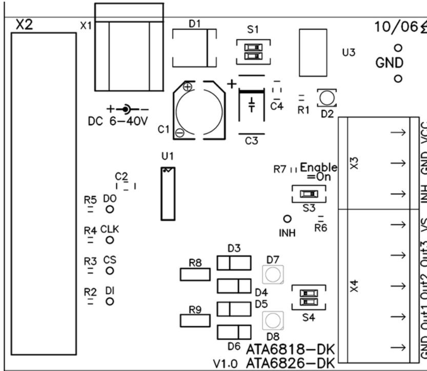
Figure 4. ATA6826-DK Design Kit, Basic Application Board Top Side, Top View
