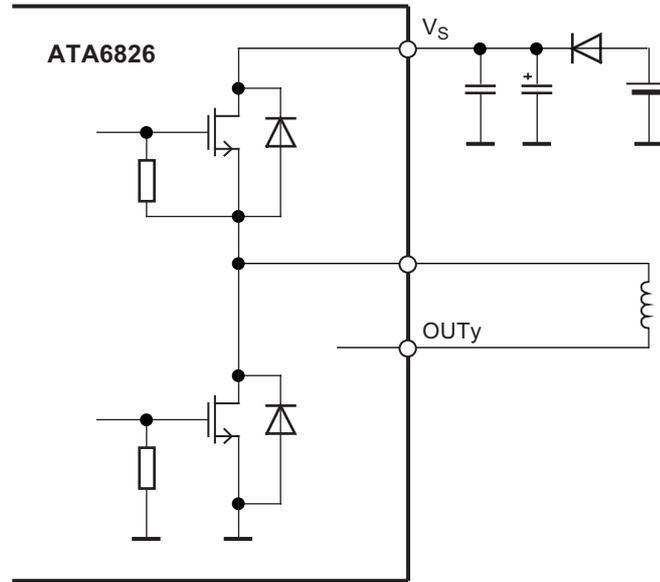
The clamping structures at the output stages limit the voltage peak and provide a path for the current after switching off. The maximum inductive shutdown energy for ATA6826 is specified as 15mJ. This value applies for both low-side and high-side outputs. The energy  $W_L$  stored in the inductor  $L$  during the switched-on state can be calculated using the following formula:
