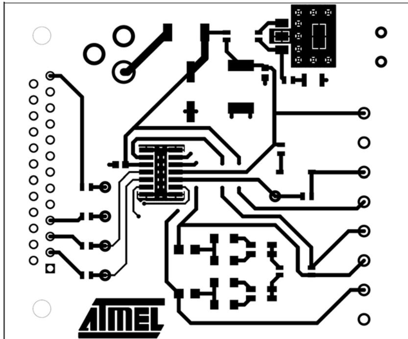
Figure 5. ATA6826-DK Design Kit, Basic Application Board; Bottom Side, Top View (as if PCB were Transparent)
