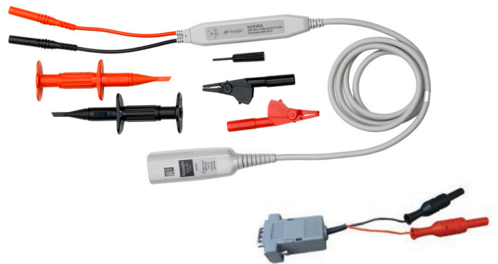
Figure 12. Keysight's N2818A 200-MHz differential active probe.
