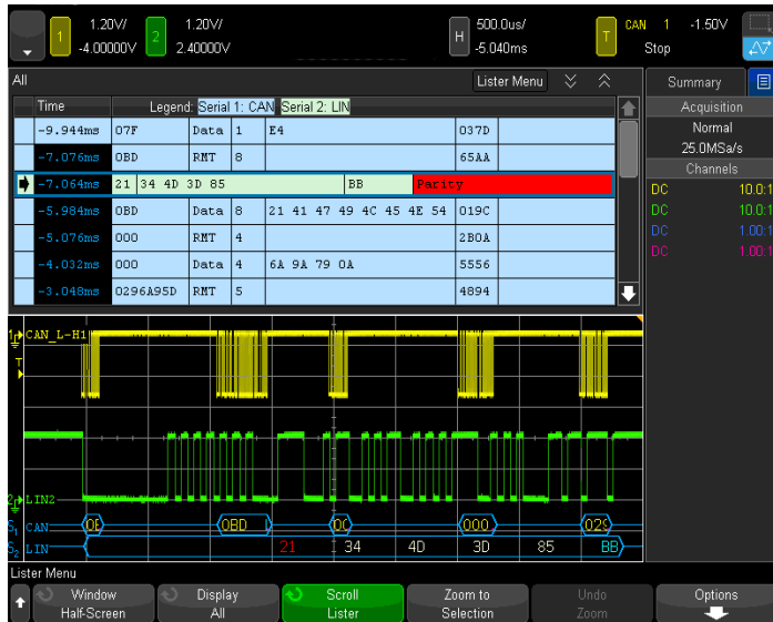
Figure 4. An interleaved “Lister” makes it easier to time-correlate activity between two decoded serial buses.
