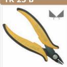
TR 25 B: Tool for a flush well finished cut. Lightweight and easy to handle with swelled blades, leaving the cut well finished. Suitable for work with plastic. Steel thickness 2.5mm. Tool length 138mm.
