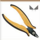
TR 30 B: Tool for a flush finished cut. Lightweight and easy to handle with swelled blades, leaving the cut well finished. Suitable for work with plastic. Steel thickness 3.0mm. Tool length 138mm
