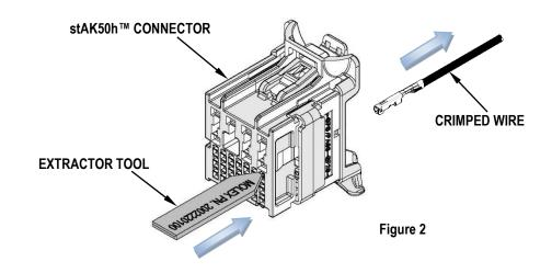
**CAUTION:** This extractor tool should be used to extract the terminal only. Using it for unintended purposes may cause injury or damage to parts. Be careful not to deform the end of the terminal.
