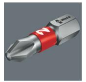
BiTorsion bits are absolutely premium products. They have a softer BiTorsion zone which reduces the hardness of the shaft by about 20 % in comparison to the drive tip. This means that the peak loads that cause bit breakage and premature wear are absorbed in this zone — something which enhances the service life of the bits.
