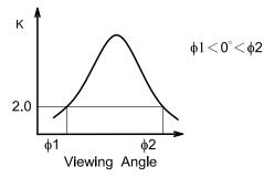
Contrast ratio K vs viewing angle  $\phi$
