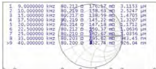
Impedance Test Ω/100 m. - start 9 KHz - stop 40 KHz.
