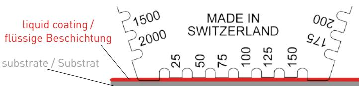
The figure shows that the tooth 100 µm (3.94 mil) has been wetted by the coating as the last tooth and that the tooth 125 µm (4.92 mil) has not been wetted. Thus, the wet film thickness of the coating is between 100 µm (3.94 mil) and 125 µm (4.92 mil).
