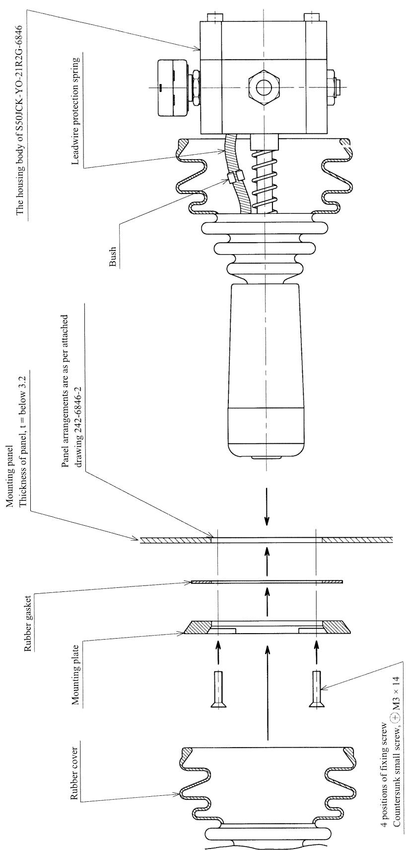
1. You can see the mounting plate when turning up rubber cover.
