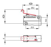
Roller lever r Actuator position Dimension 🕐 in mm Lever length 22.6 Free position  $22.4 \pm 0.3$ Operating position  $21.1 \pm 0.4$ Release position  $21.4 \pm 0.4$ Total positive opening travel 19.3 19.0 Total travel position Movement differential 0.3 (between operating and (typical) release position)
