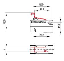
• Simulated roller lever, long Actuator style **v**
