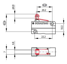
Simulated roller lever, medium Actuator style u
