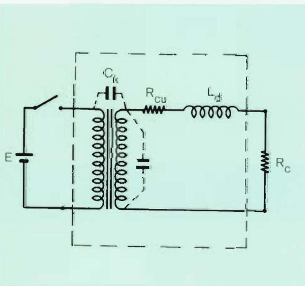
Insulation transformers, designed for triacs or thyristor firing, need the following characteristics:
