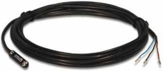
The P1D sensors can easily be installed from the side in the sensor groove, at any position along the piston stroke. The sensors are completely recessed and thus mechanically protected. Choose between electronic or reed sensors and several cable lengths and 8 mm and M12 connectors. The same standard sensors are used for all P1D versions.
