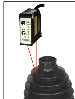
Measuring CV Joint Deflection
